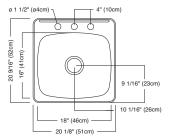
23SB.202083.290 Standard drilling: 3 hole
